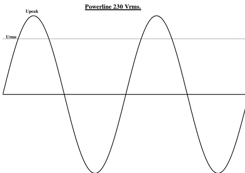
This sine wave is showing the output from the power line in your house. Oscillators used in radio frequency circuits are always very low power devices, in contrast to AC generators in power stations. Nevertheless, the AC power generator and the electronic are related, in that they both produce sinusoidal output.
