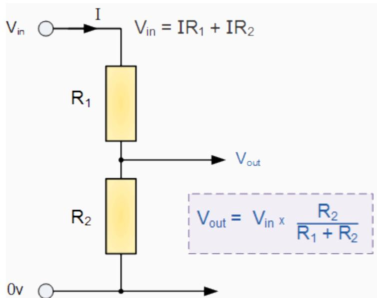
In this circuit the two resistors are connected in series across  $V_{in}$ , which is the power supply voltage connected to the resistor,  $R_1$ , where the output voltage  $V_{out}$  is the voltage across the resistor  $R_2$  which is given by the formula. If more resistors are connected in series to the circuit then different voltages will appear across each resistor with regards to their
