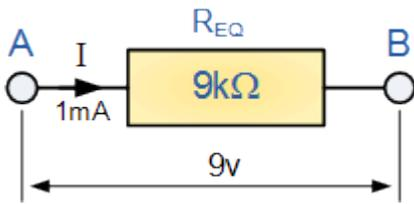
So we can replace all three individual resistors above with just one single equivalent resistor which will have a value of  $9k\Omega$ .
