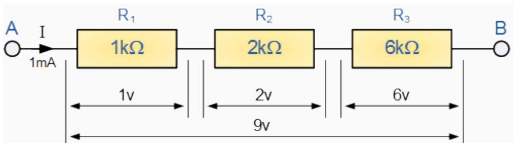
As the resistors are connected together in series the same current passes through each resistor in the chain and the total resistance,  $R_T$  of the circuit must be **equal** to the sum of all the individual resistors added together. That is
