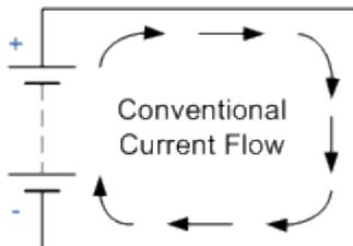
Conventionally this is the flow of positive charge around a circuit. The diagram at the left shows the movement of the positive charge (holes) which flows from the positive terminal of the battery, through the circuit and returns to the negative terminal of the battery. This was the convention chosen during the discovery of electricity in which the direction of electric current was thought to flow in a circuit. In circuit diagrams, the arrows shown on
